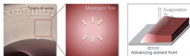
Fig. 1 Representative photograph shows the uniform coating of red wine at macroscale enabled by the Marangoni flow. The dissimilar evaporation rates between each solvent result in advancing solvent fronts toward un-wetted areas.
